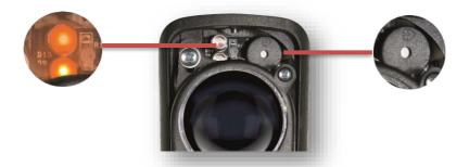
• Orient the TX optic on the column towards the RX optic, vertically and horizontally acting as explained above, until you find the maximum alignment.
