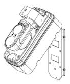
Following the calibration and verification of correct operation, replace the cover and secure it with the closing screw located on the lower side of the device.
