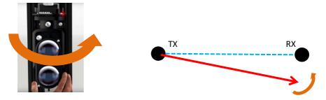
• The maximum alignment condition will be reached when the high-intensity LEDs are on steady and the buzzer will emit a continuous sound, for this reason, it may be necessary to make minor adjustments also on the RX optic.
